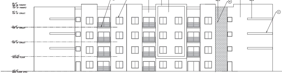
BLDG 1 INTERIOR EAST ELEVATION (BLDG 2 SIM. REVERSED) 1/8" = 1'-0"
