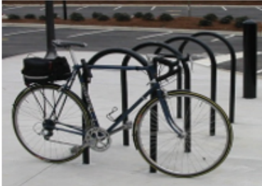
Inverted-U bicycle rack, where both ends of the “U” reach the ground.
