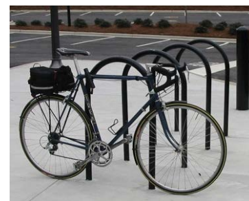
Inverted-U bicycle rack, where both ends of the "U"
