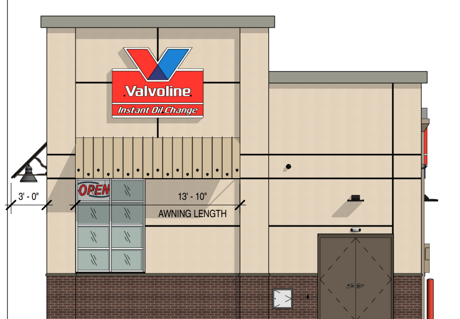
2 OVERALL RIGHT SIDE EXTERIOR ELEVATION (RIGHT) Scale: 1/8" = 1'-0"
