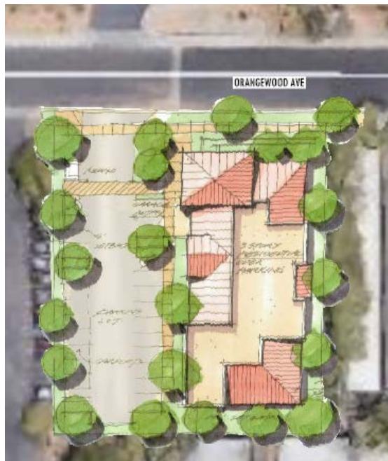
Conceptual plan showing residential units (over parking) on the east and surface parking on the west.
