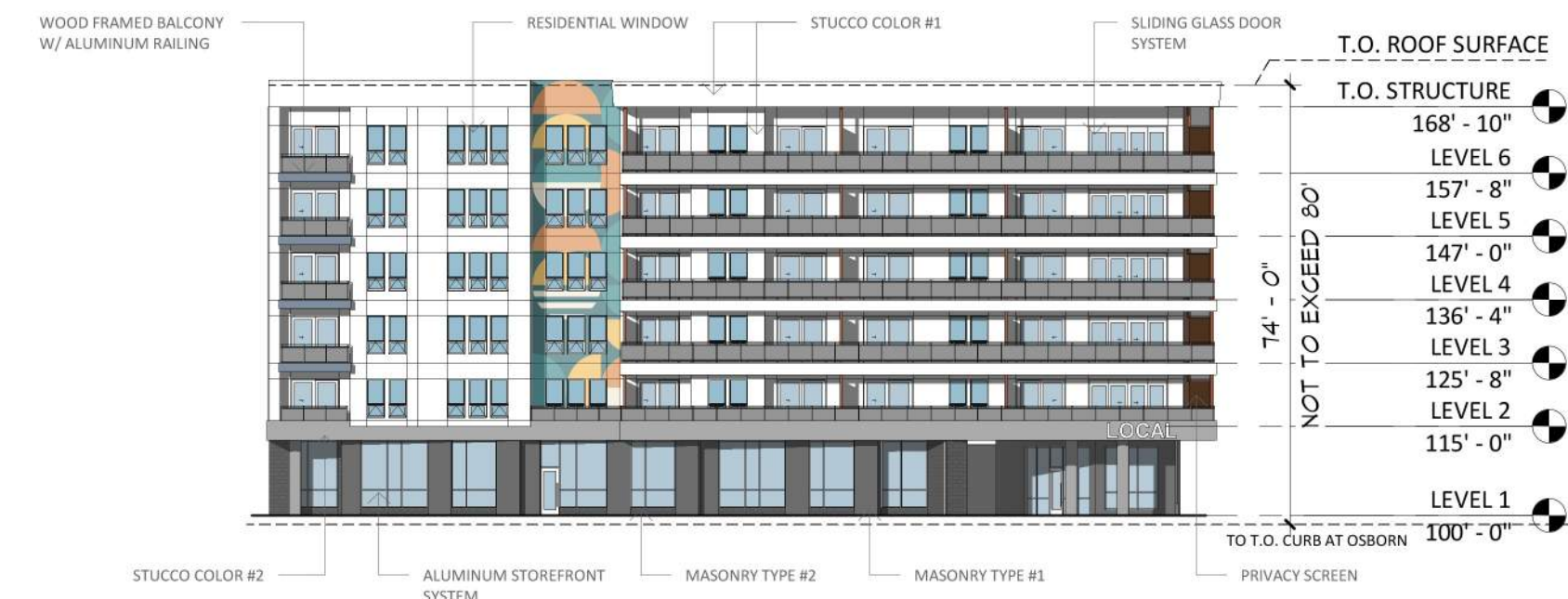
2 BUILDING ELEVATION - OVERALL SOUTH 1" = 30'-0"
