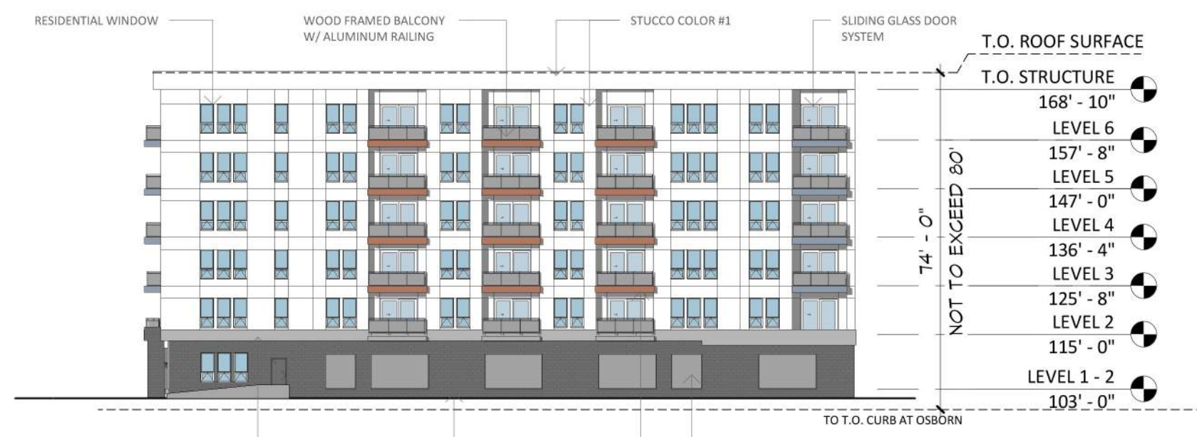
4 BUILDING ELEVATION - OVERALL NORTH 1" = 30'-0"
