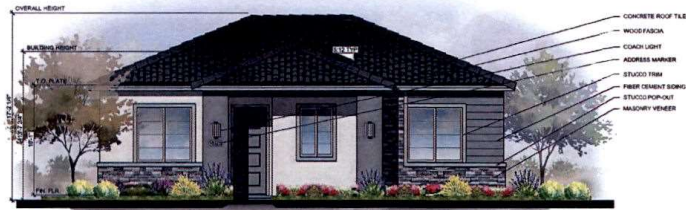
PLAN 2 PERIMETER UNITS FRONT ELEVATION ELEVATION B 1/8" = 1'-0"
