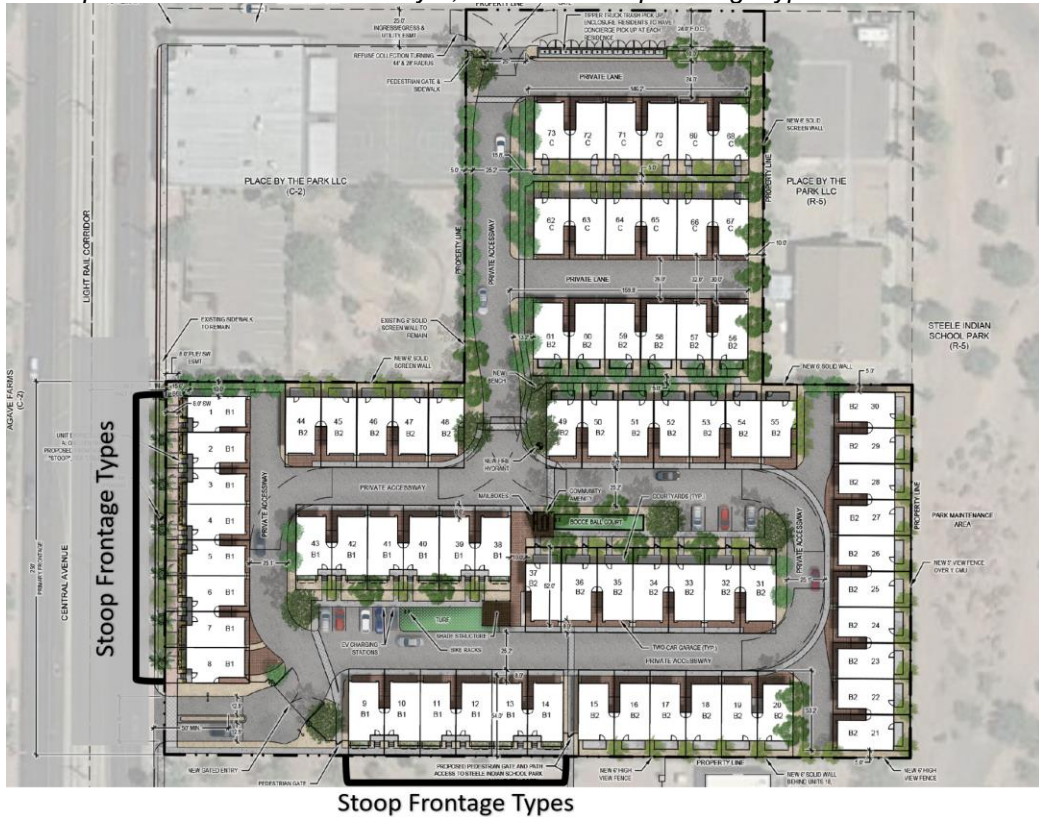
Conceptual Site Plan from February 1, 2022 with stoop frontage types annotated. Source: Norris Design
