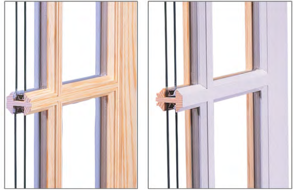
The dual-pane replacement windows shown above have true divided lights, with the muntins extending all the way through the glass. This type of window is recommended because it closely replicates the look of a historic window.
